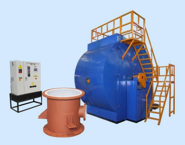
Vinodrai Engineers has developed a range of special rotational moulding machine most suitable for Rotolining application. The rotolining process allows for a seamless polymer coating to be applied to the interior surfaces of metal vessel, pipeline, pipe fittings or any hollow metal structure to protect against corrosion and abrasion in chemical services.
