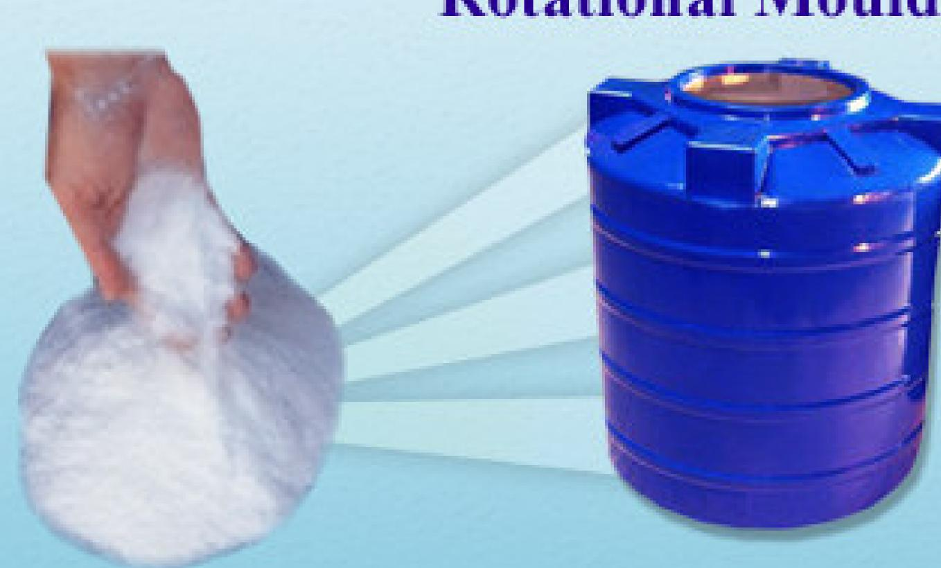
Rotational moulding needs resin in powder form. The particle size, shape and particle size distribution is measure of powder quality. Powder quality plays a very important role in rotational moulding. Following are the resultant effects of the good quality powder. Optimization of charge weight to meet rising compitition.
